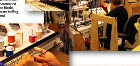
eventually reel seats, cork handles and guides were attached. At this point rods were nearing completion. We watched as workers applied epoxy finish on wraps and guides then placed on large rotators until the applied finish hardened.
